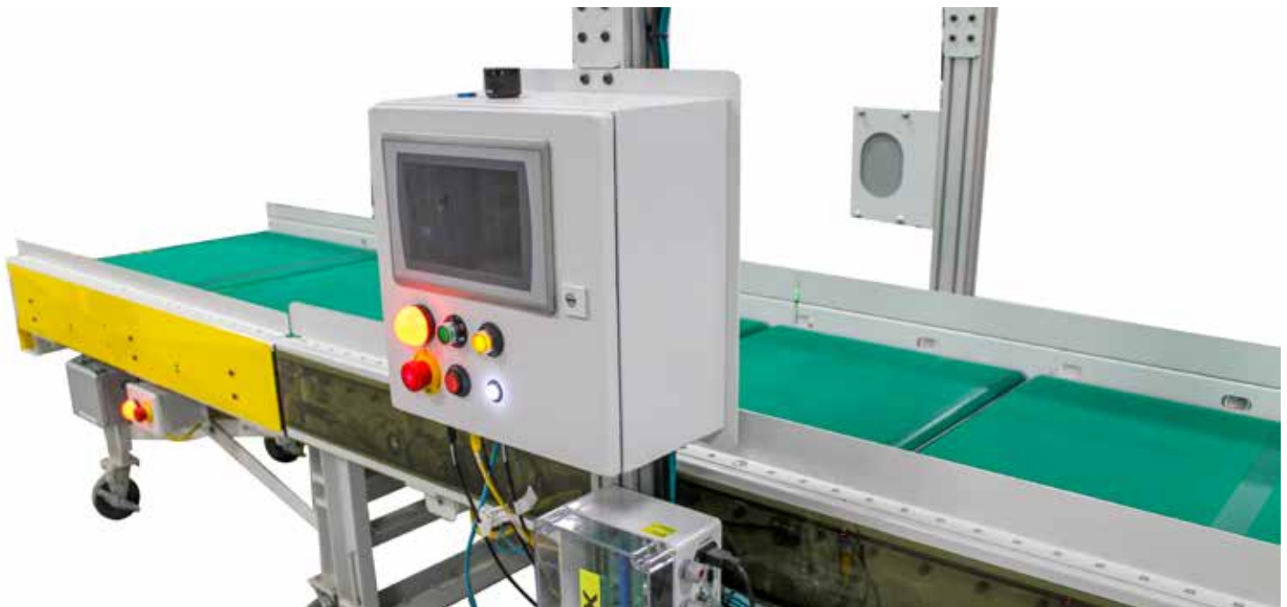
HMI control panel
